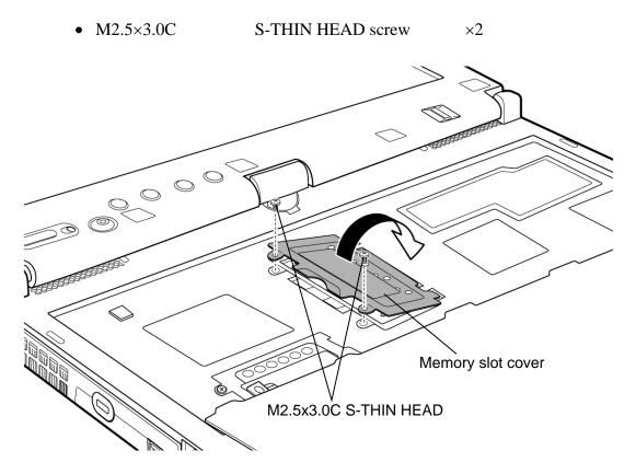
Figure 4-18 Removing the memory slot cover (slot A)
